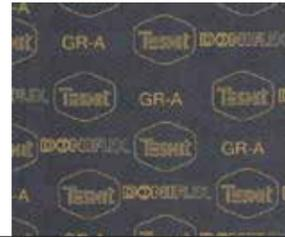
Soft sealing material reinforced with tanged steel insert. Excellent thermal and stress resistance combined with very good adaptability to flange irregularities.
